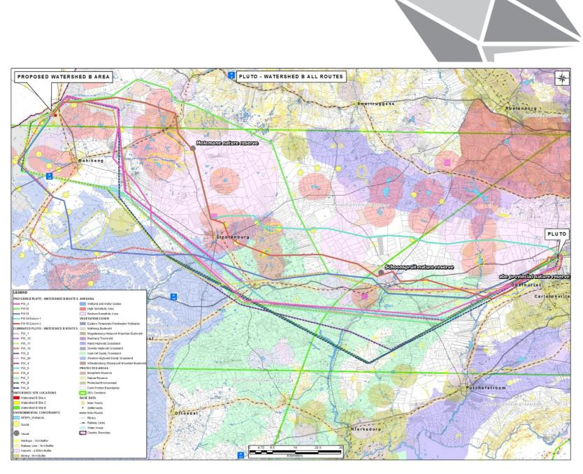
Figure 3. All route options between Pluto and Watershed B substation, based on the outcomes of the route screening process
